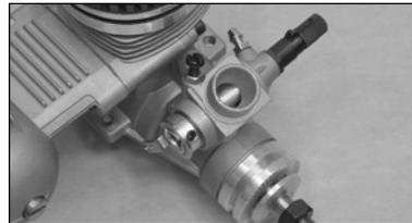
also adjusts the closure of the throttle barrel. We recommend adjusting the idle stop screw to allow the throttle barrel to close completely. This will allow you to adjust the idle speed via your transmitter; therefore, you will
