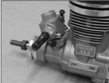
the base of the carburetor into the crankcase, being careful to keep the carburetor perpendicular to the front of the engine. Using your thumb, push down firmly on the carburetor so that the base of the carburetor sets completely into the crankcase. An o-ring is installed on the carburetor throat to seal the joint. While holding the
