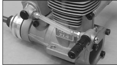
To mount the rear needle valve assembly, use an adjustable wrench to unscrew and remove the needle valve assembly from the carburetor and to unscrew and remove the plug from the rear needle valve mount.
